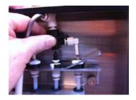
Push the parts together and turn the upper part counter clockwise.
