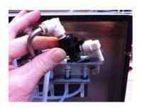
Press the grey lock and remove the tubes.
