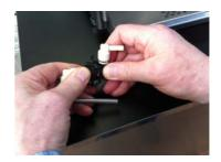
Lift outlet tube locking lever.
