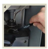
Brush around the top of the brew unit, using the long handled brush in order to remove any ground coffee deposits.
