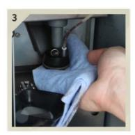
Thoroughly wipe underneath the piston cleaning the metal filter and wipe all around cleaning the O-ring, to remove deposits of coffee. Finish with cleaning the metal filter on the bottom piston.
