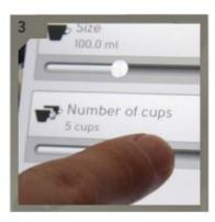
Slide the number of cups up to 5 and select "Start now". The machine will run the cleaning liquid through the system and clean the milk foamer.
