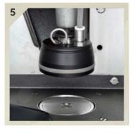
The stainless steel cylinder top must be completely clean with no coffee remains. Push the scraper arm back in place.
