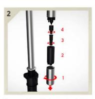
Remove the milk foamer by twisting the metal head anti-clockwise. Slide down the black casing. Unscrew the black foaming heads. Clean in warm water to ensure all milk deposits are removed. Dry & reattach.
