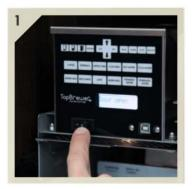
Open the stainless door, wait until the piston raises. Turn off the Top-Brewer using the on/off button on the front panel of the machine.
